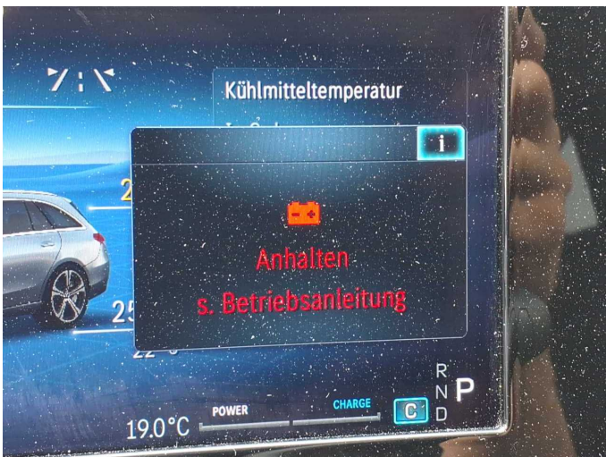
Damage 2: Electrical system: Battery - Empty - Perform diagnosis
