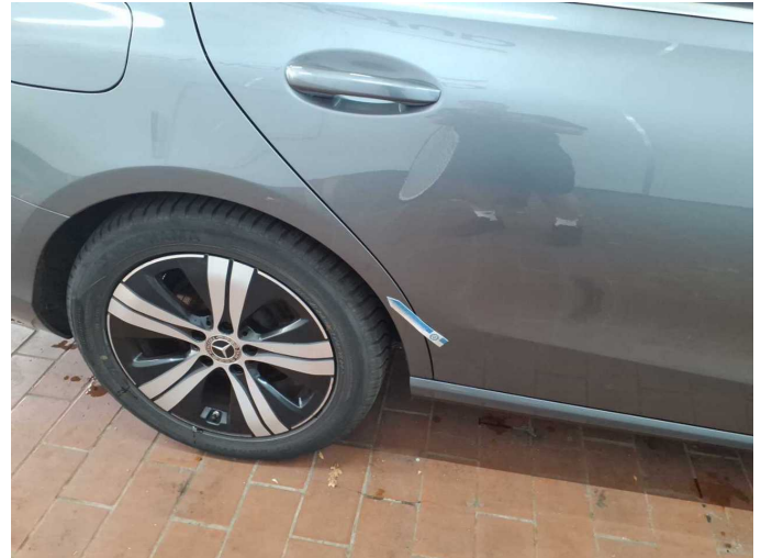
Damage 4: Side panel - rear right side: Elbow - dent(s) - Clean
