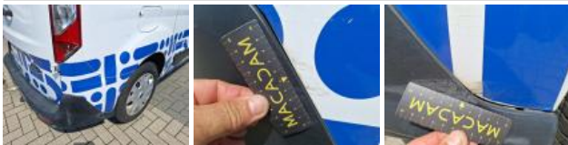
Boot door panel RL, Dent(s), Acceptable
