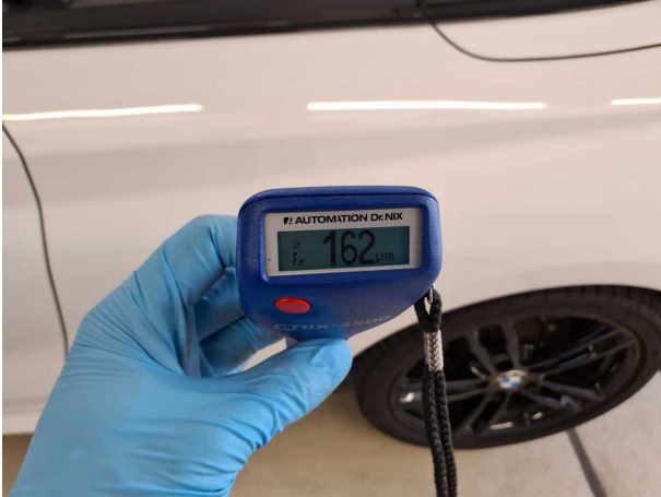
Repainting 1: Side panel - rear left side, Door - front left side
