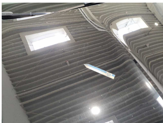
Damage 2: Bonnet: Bonnet - Scratch(es) - Smart repair
