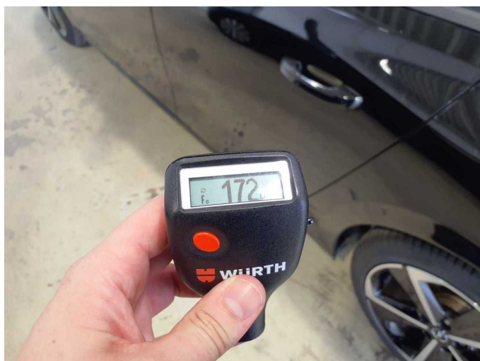
Repainting 2: Door - rear left side
