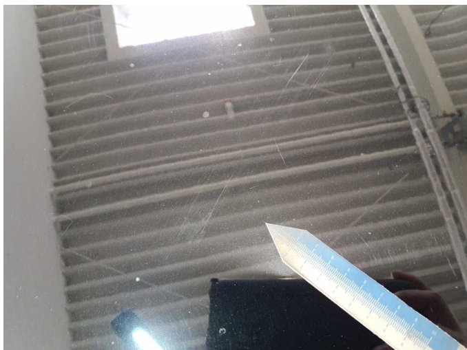
Damage 2: Bonnet: Bonnet - Scratch(es) - Smart repair
