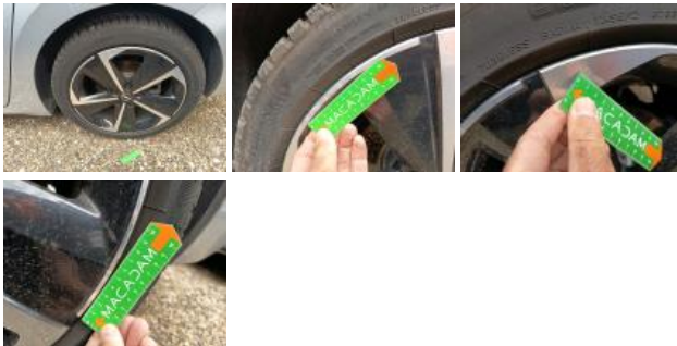
Tyre FR, Out of tolerance, Replace
