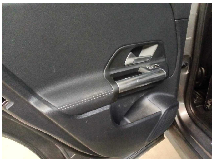
Damage 3: Door - rear left side: Handle - Scratch(es) - Smart repair
