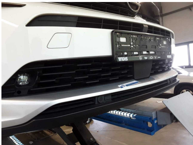
Wear and tear 5: Front bumper: Spoiler - Scratch(es) - No deduction
