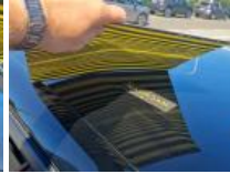
Roof, Dent(s), Paintless dent repair
