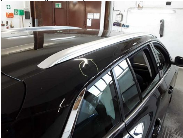
Damage #11: Roof: Roof rail - right side - Dent / paintcoat damage - Repair and paint
