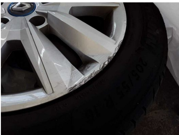
Damage #3: 2nd wheel set: Wheel cover set - complete - Scratch... - Replace
