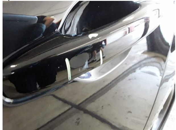
Damage #8: Door - rear left side: Door handle - outside - Scratched - Smart repair
