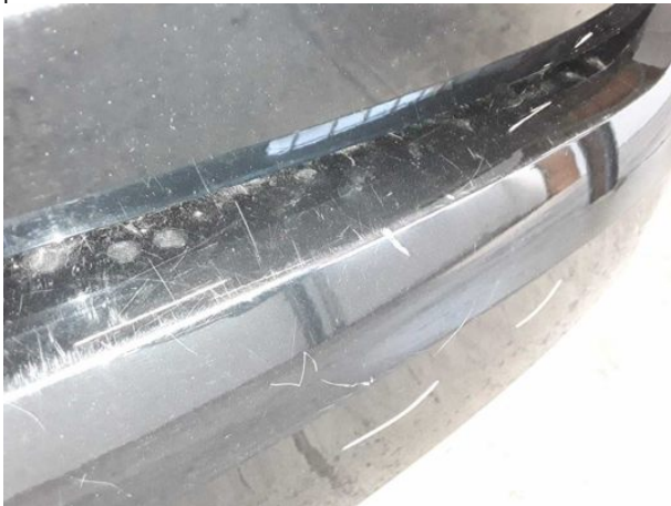
Damage #12: Rear bumper: Rear bumper - Scratched - Repair and paint
