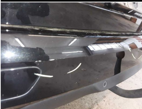
Damage #12: Rear bumper: Rear bumper - Scratched - Repair and paint
