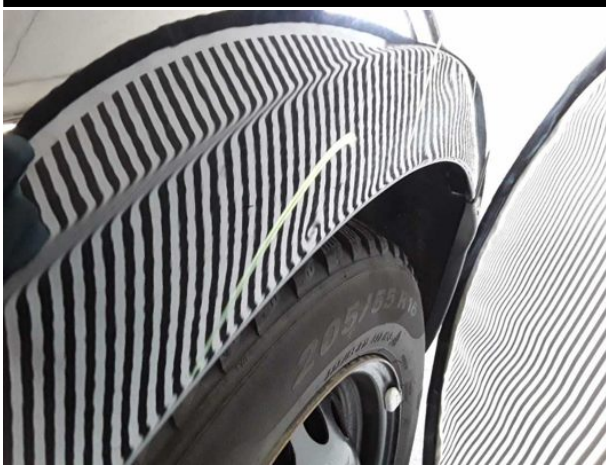
Damage #10: Side panel - rear left side: Side panel - Dent / paintcoat damage - Smart repair
