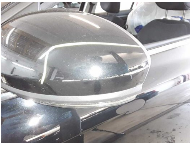
Damage #9: Wing mirror - left side: Cap - Scratched - Smart repair
