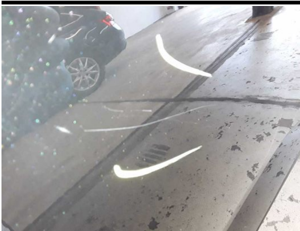
Damage #13: Door - rear left side: Door - Scratched - Repair and paint
