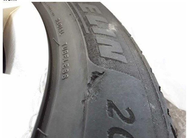
Damage #6: 2nd wheel set: 1 tyre - Damaged - Replace
