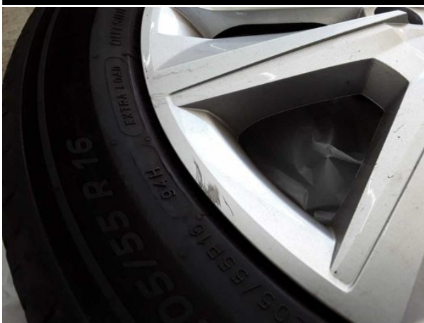
Damage #3: 2nd wheel set: Wheel cover set - complete - Scratch... - Replace
