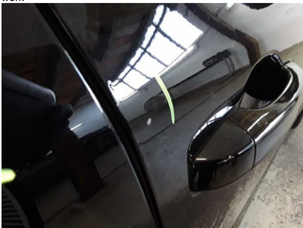
Damage #5: Door - front right side: Door - Scratched - Smart repair
