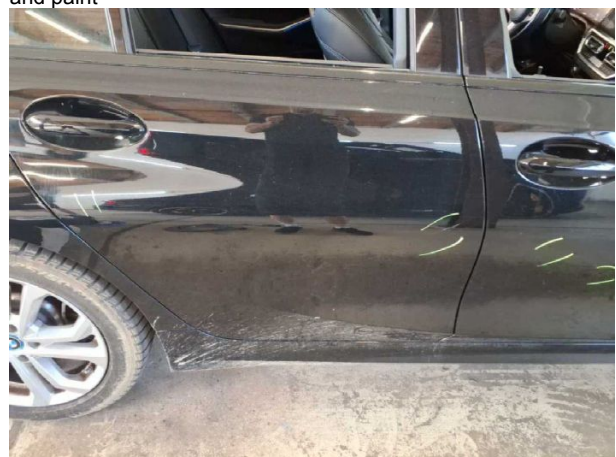
Damage #6: Door - rear right side: Door - Scratched - Repair and paint
