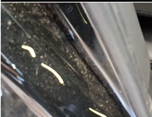
Damage #3: Side panel - rear right side: Sill - Scratched - Cover / polish
