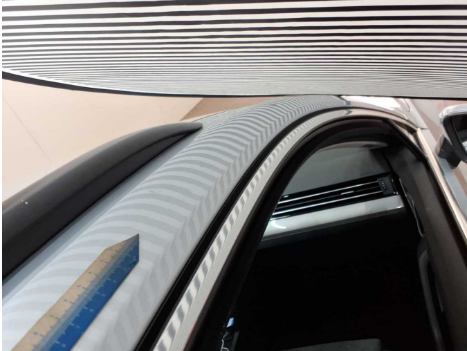
Damage 3: Roof: Roof rail - right side - dent(s) - Smooth repair work
