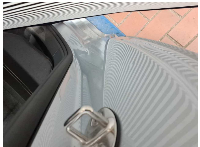
Damage 5: Side panel - rear right side: Sill (Kratzer) - dent(s) - Smart repair
