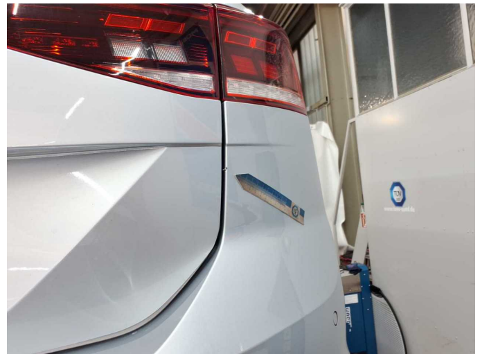
Damage 6: Rear bumper: Rear bumper - Scratch(es) - Paint
