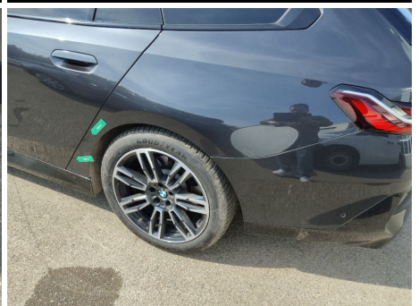
Kotflügel / Hinten Links / Delle
