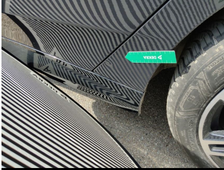
Kotflügel / Hinten Links / Delle
