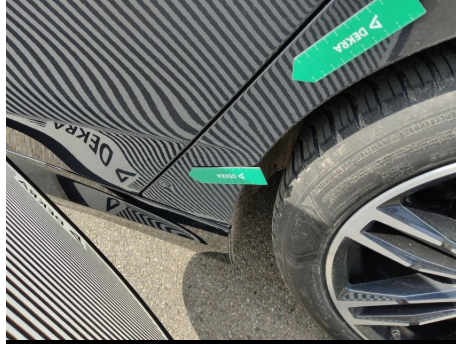
Kotflügel / Hinten Links / Delle
