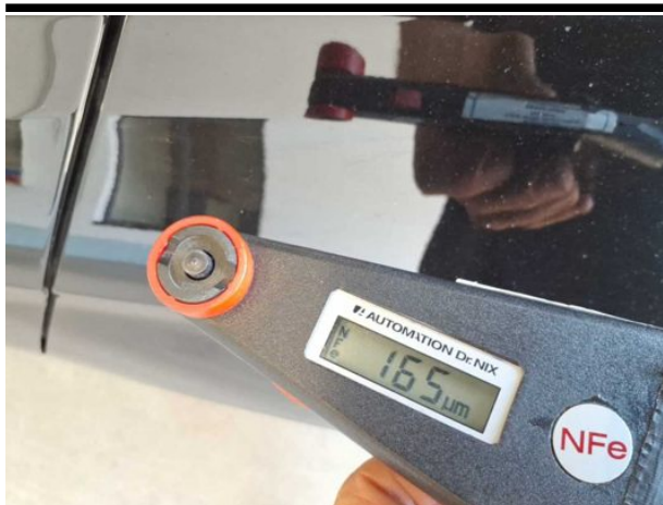
Repainting 1: Roof rail - left side, Roof rail - right side, Mudguard - left side, Mudguard - right side, Side panel - rear left side, Door -
