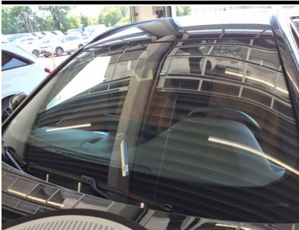
Damage #5: Vehicle glazing: Windscreen with lane departure assistant - Stone chips - Replace
