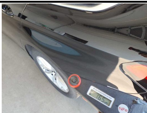
Repainting 1: Roof rail - left side, Roof rail - right side, Mudguard - left side, Mudguard - right side, Side panel - rear
