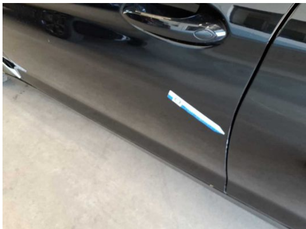
Damage #1: Door - front left side: Door edge - Scratch(es) - Cover / polish
