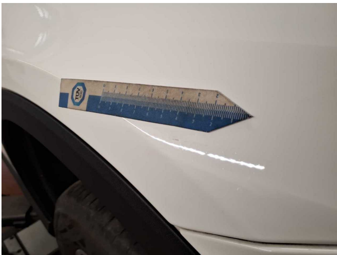
Wear and tear 4: Mudguard - right side: Mudguard - right side - Scratch(es) - No deduction
