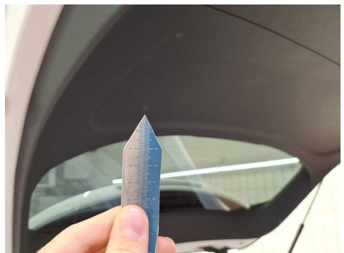
Wear and tear 5: Trim / covers: Boot lid - interior trim - Scratch(es) - No deduction
