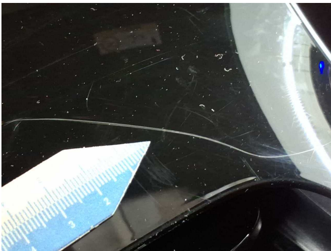
Damage 1: Instrument panel: Centre console - front - Scratch(es) - Loss in value
