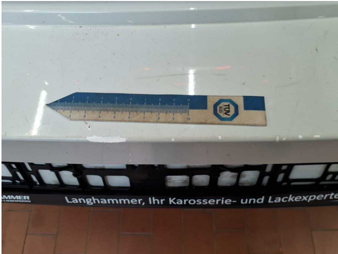
Damage 11: Rear bumper: Rear bumper - Scratch(es) - Paint
