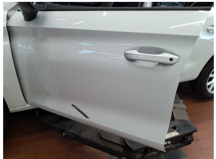
Damage 12: Door - front left side: Door - Corrosion - Repair and paint
