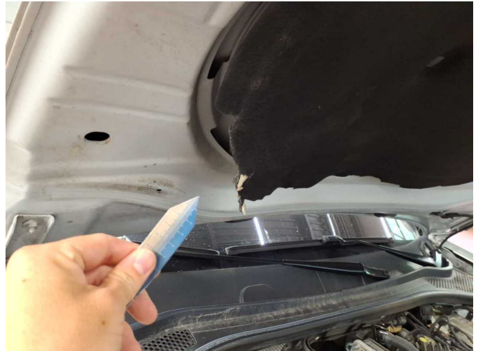
Damage 3: Bonnet: Insulation lining - Broken / torn - Replace
