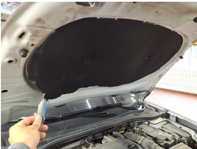
Damage 3: Bonnet: Insulation lining - Broken / torn - Replace
