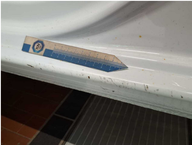
Damage 8: Sill - left side: Sill - Corrosion - Paint
