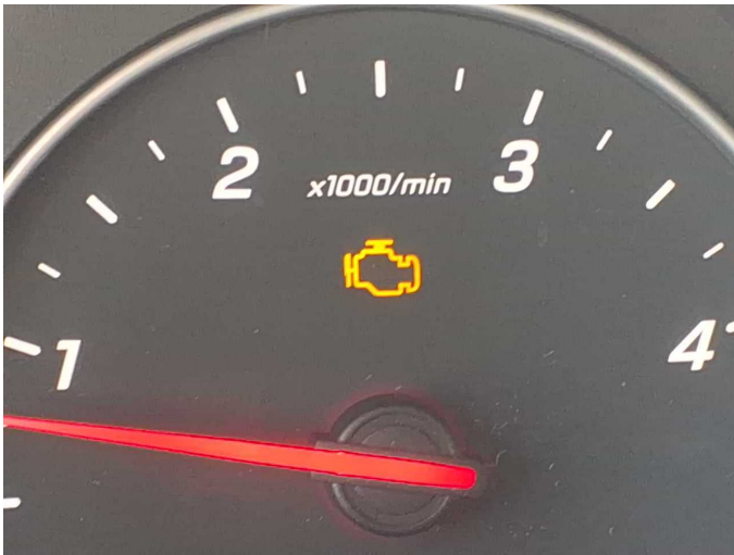
Damage 1: Instrument panel: Indicator light (Motorkontrolle) - on - Perform diagnosis
