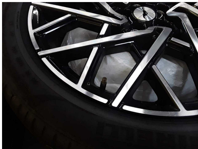
Damage 1: Wheel / tyres: Valve (Kappe) - Missing - Replace
