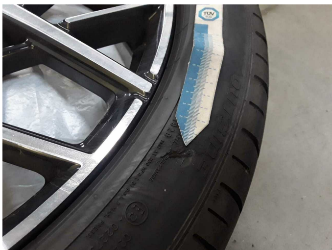
Damage 4: 2nd wheel set: 1 tyre - Damaged - Replace
