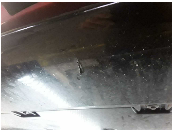
Damage 2: Front bumper: Spoiler (Windabweiser vorne) - Scratched - Smart repair
