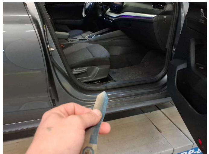
Damage 3: Body: Door seal - front right side - Broken / torn - Replace
