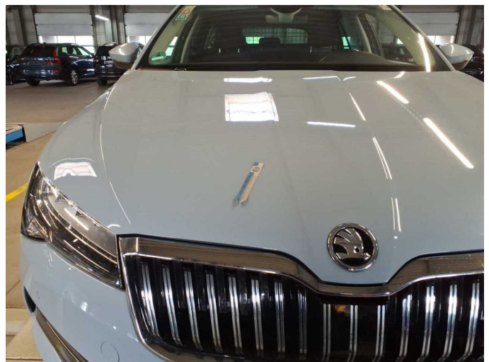
Damage 4: Bonnet: Bonnet - dent(s) - Smooth repair work
