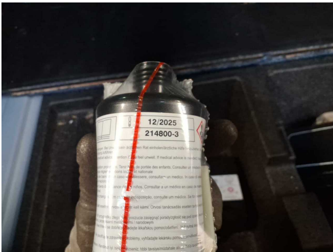
Damage 1: Equipment: Tirefit filler - Expired - Replace
