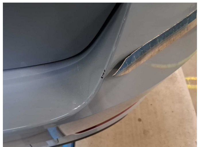
Damage 6: Rear bumper: Rear bumper - Scratch(es) - Paint
