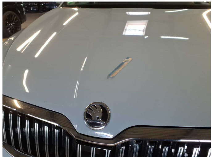
Damage 4: Bonnet: Bonnet - dent(s) - Smooth repair work
