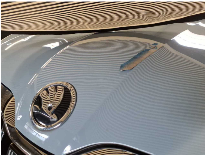
Damage 4: Bonnet: Bonnet - dent(s) - Smooth repair work
