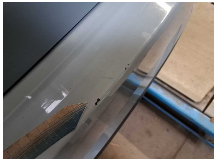
Damage 6: Rear bumper: Rear bumper - Scratch(es) - Paint
