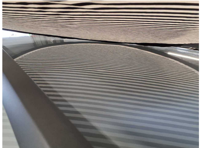
Damage 5: Roof: Roof - dent(s) - Smooth repair work
