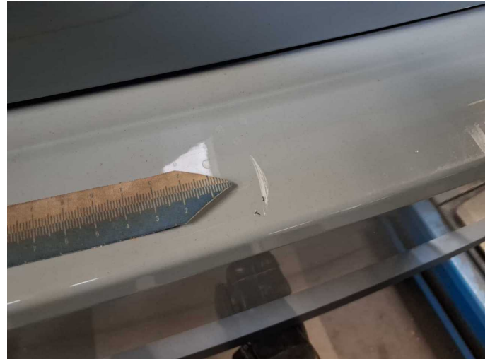
Damage 6: Rear bumper: Rear bumper - Scratch(es) - Paint
