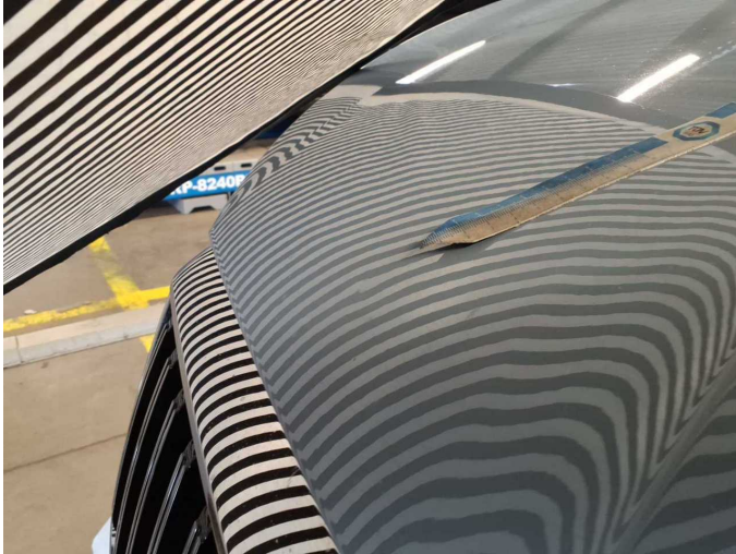
Damage 4: Bonnet: Bonnet - dent(s) - Smooth repair work
