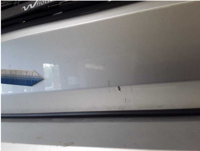
Damage 5: Boot lid / rear door: Boot lid - Scratch(es) - Paint
