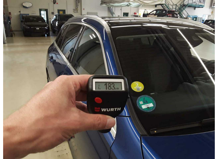
Roof rail - right side: 183 µm
