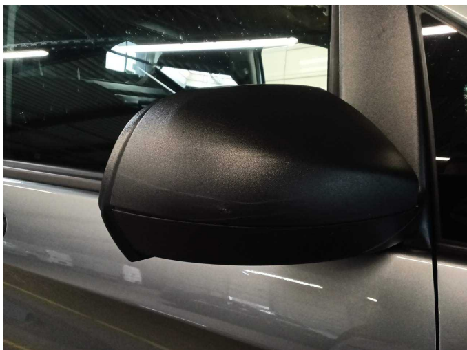
Wear and tear 1: Wing mirror - right side: Mirror housing - Scratch(es) - No deduction
