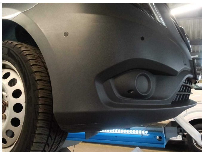
Damage 9: Front bumper: Front bumper (unpainted) - Scratched - Replace
