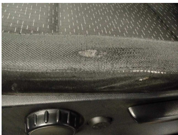
Damage 7: Seat - front: Seat cover - left side - Damaged - Replace
