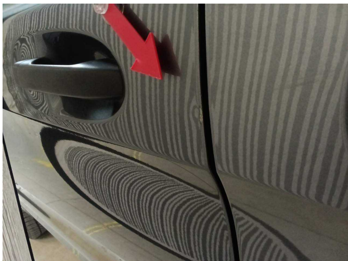
Damage 10: Sliding door, right: Sliding door - Dent / paintcoat damage - Repair and paint
