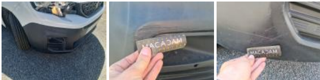
Bumper F, Scratch(es), Repair and paint (complete)
