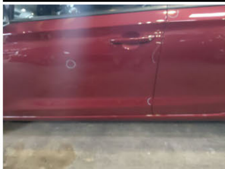
Tür / Vorne Links / Kratzer
