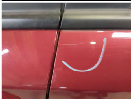
Tür / Hinten Links / Kratzer
