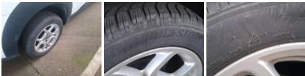
Tyre RL, Out of tolerance, Replace
