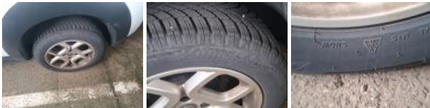
Tyre FL, Out of tolerance, Replace
