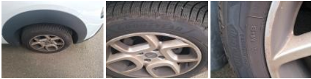
Tyre RR, Out of tolerance, Replace
