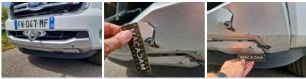
Grille, Broken, Replace
