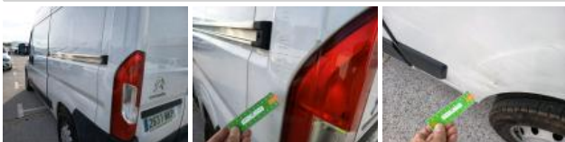
Sliding door L, Dent(s) and scratch(es), Repair and paint (complete)
