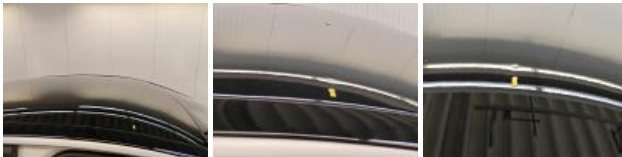
Roof, Dent(s), Repair and paint (complete)
