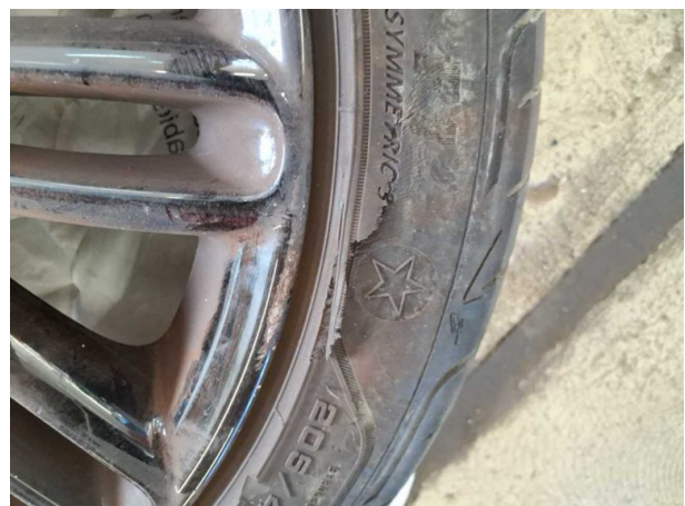
Damage #5: 2nd wheel set: 1 tyre - Damaged - Replace
