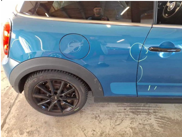
Damage #10: Side panel - rear right side: Side panel - Scratched - Repair and paint
