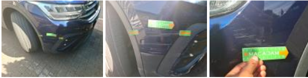
Bumper moulding F, Scratch(es), Replace
