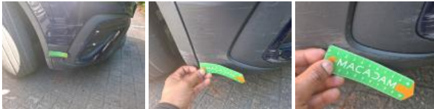
Bumper moulding F, Scratch(es), Replace
