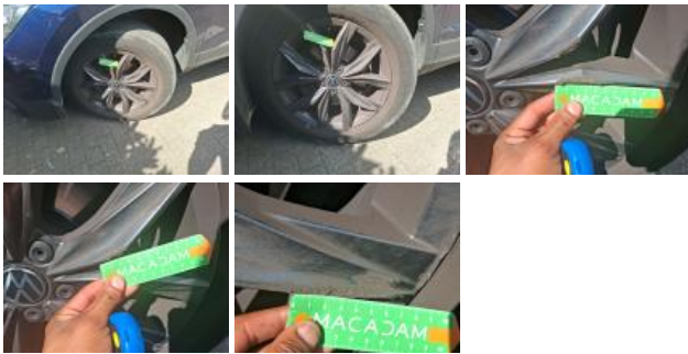
Tyre FR, Out of tolerance, Replace
