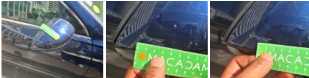
Door RR, Dent(s), Repair and paint (complete)
