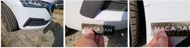
Bumper moulding FR, Scratch(es), Replace
