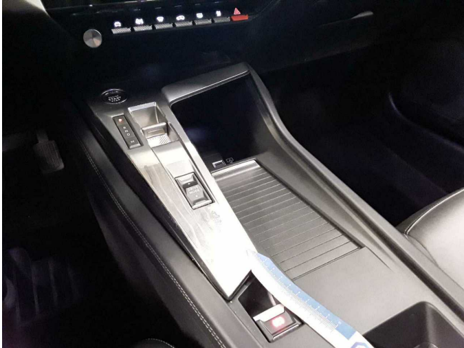
Damage 3: Instrument panel: Centre console - front - Scratched - Replace
