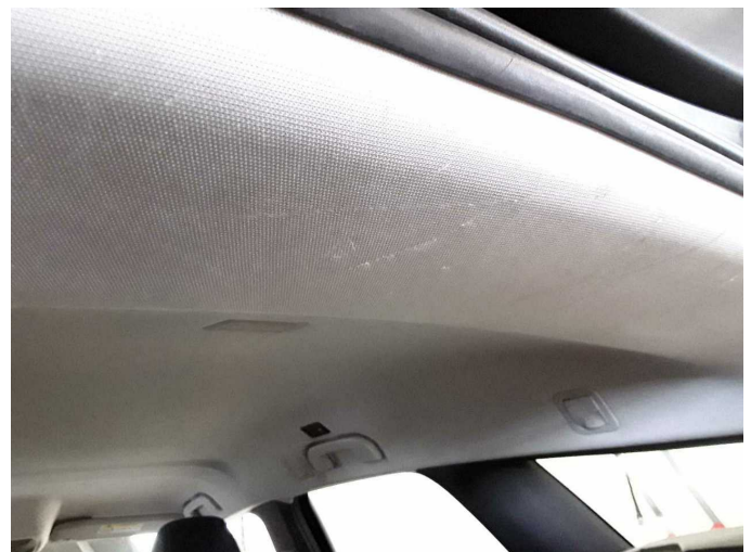
Damage 2: Trim / covers: Roof lining - Scratched - Loss in value
