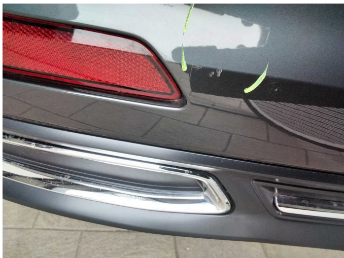
Damage 6: Rear bumper: Rear bumper - Scratch(es) - Paint
