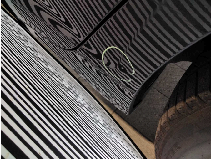
Damage 3: Side panel - rear left side: Side panel - dent(s) - Smart repair
