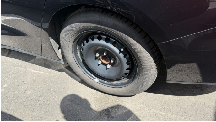
Damage 4: Wheel / tyres: Wheel cover - rear left side - Missing - Replace
