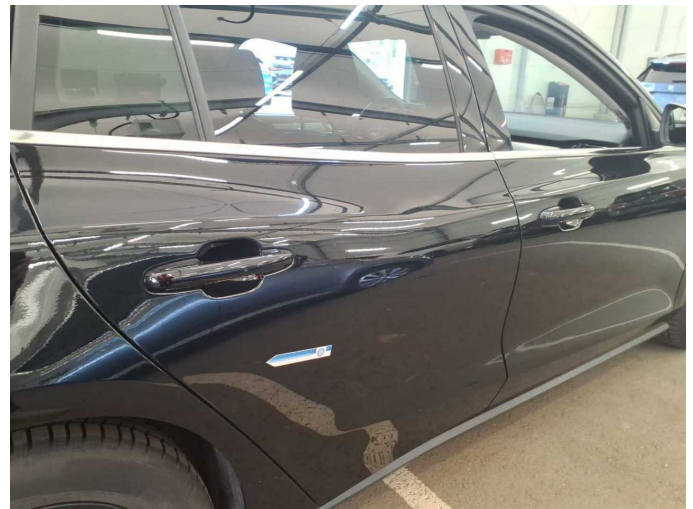
Damage 9: Door - rear right side: Door - Scratch(es) - Smart repair
