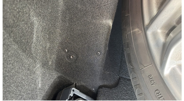
Damage 11: Trim / covers: Cargo area - lining -left side - Differs from the original configuration - Replace
