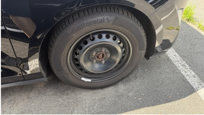
Damage 1: Wheel / tyres: Wheel cover - front right side - Missing - Replace
