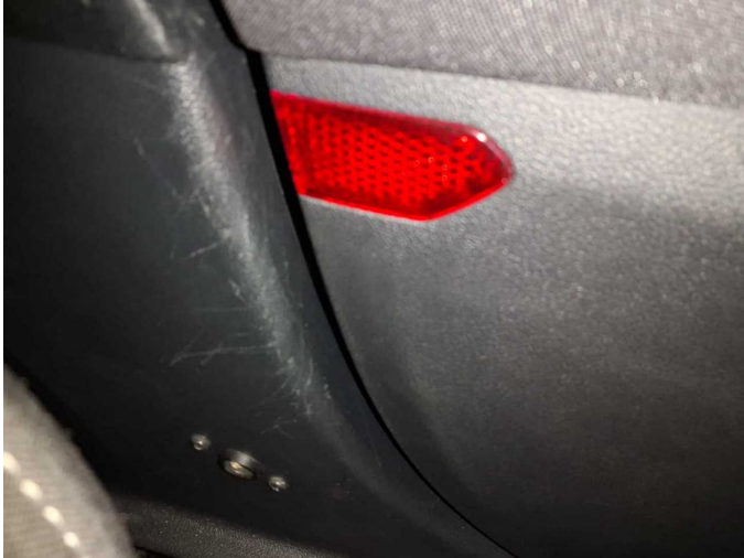
Damage 7: Trim / covers: B-pillar - trim - interior, left side (Fehlbohrungen) - Differs from the original configuration - Replace
