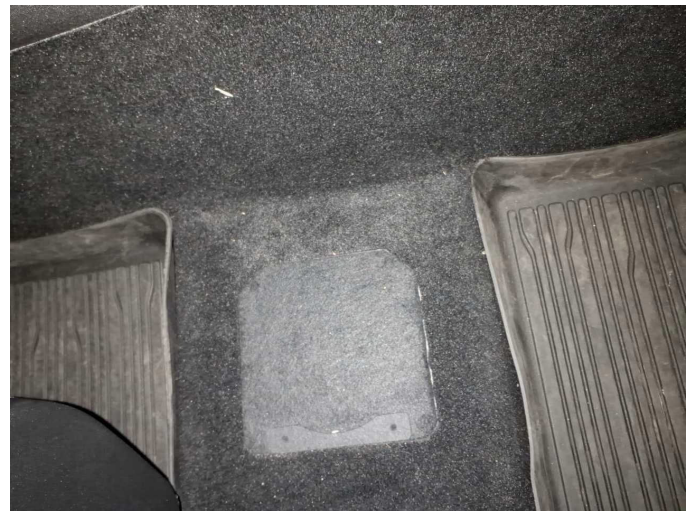
Damage 13: Trim / covers: Carpet - Differs from the original configuration - Replace
