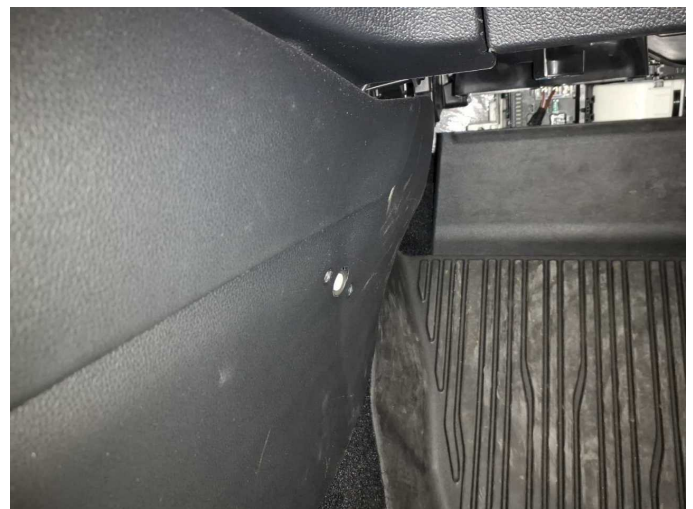
Damage 10: Instrument panel: Centre console - front (Blende Rechts, Fehlbohrungen) - Differs from the original configuration - Replace
