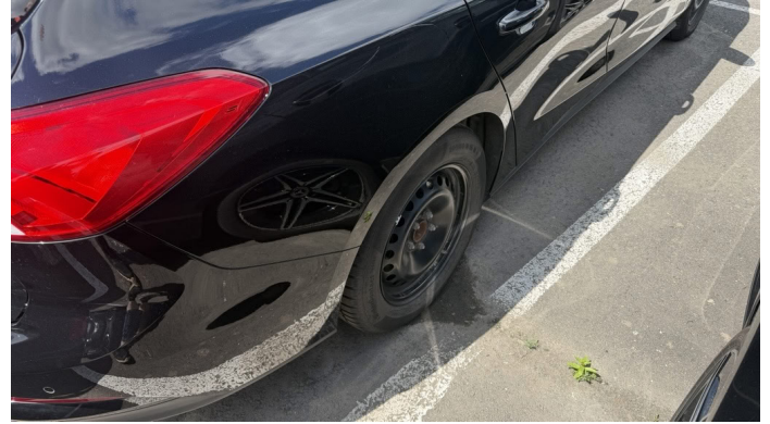
Damage 2: Wheel / tyres: Wheel cover - rear right side - Missing - Replace
