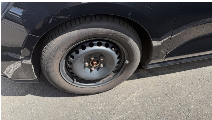
Damage 3: Wheel / tyres: Wheel cover - front left side - Missing - Replace
