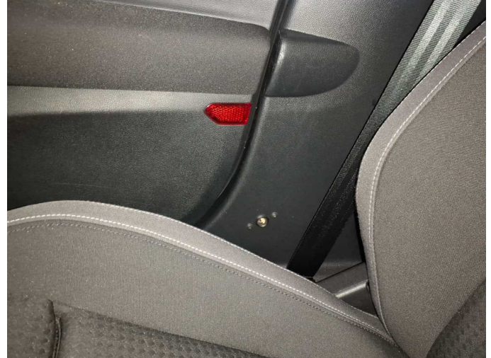
Damage 8: Trim / covers: B-pillar - trim - interior, right side (Fehlbohrungen) - Differs from the original configuration - Replace
