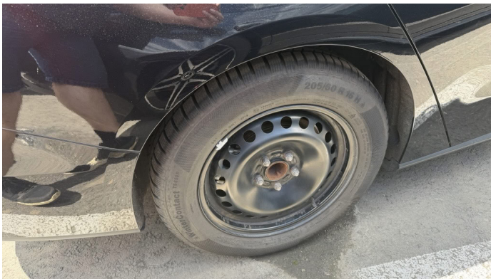
Damage 2: Wheel / tyres: Wheel cover - rear right side - Missing - Replace
