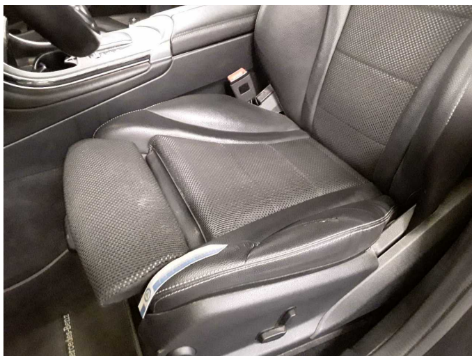
Wear and tear 6: Seat - front: Seat cover - left side - Porous / cracked - No deduction
