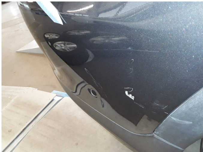
Damage 4: Rear bumper: Rear bumper - Scratched - Paint
