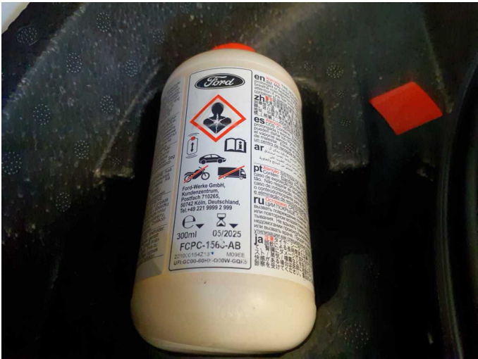
Damage 1: Equipment: Tirefit filler - Expired - Replace
