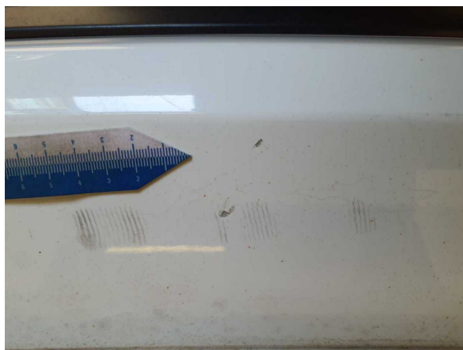
Damage 6: Rear bumper: Rear bumper - Scratch(es) - Paint
