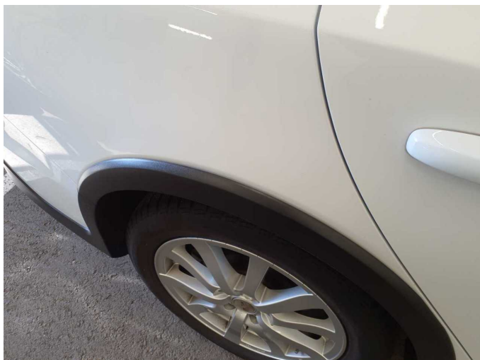
Damage 2: Side panel - rear right side: Wheel well extension - Malposition - Un- / install
