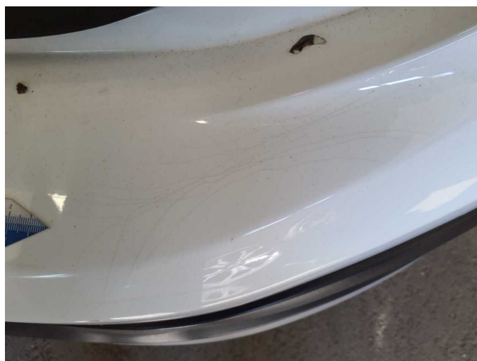
Damage 6: Rear bumper: Rear bumper - Scratch(es) - Paint
