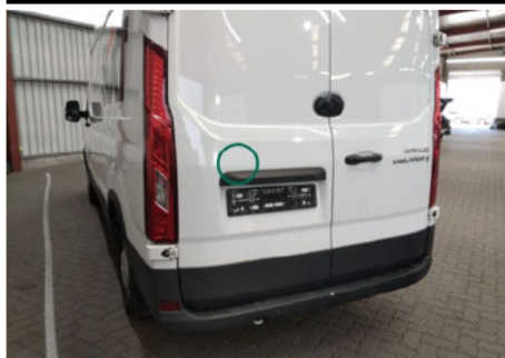
Heckklappe / Kofferraumtür / Unten Links / Delle
