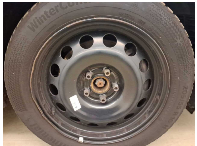
Damage 2: Wheel / tyres: Wheel rim - front right side - Deformed - Replace
