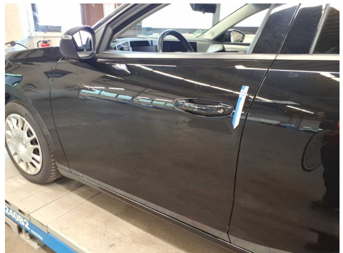
Damage 3: Door - front left side: Door edge - Scratched - Smart repair
