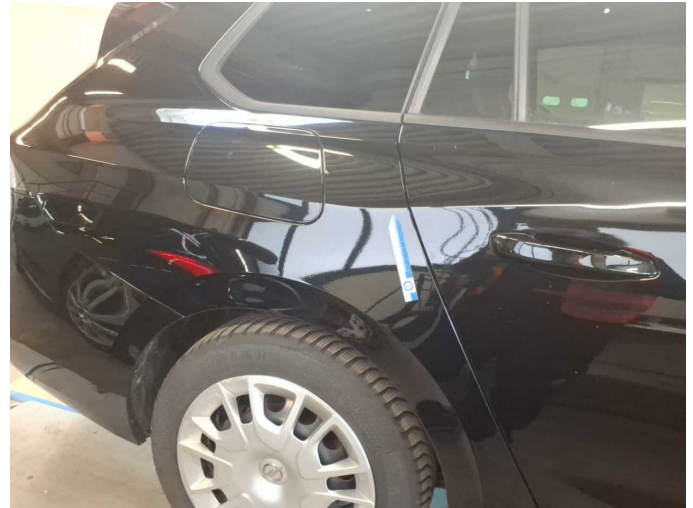
Damage 4: Side panel - rear right side: Side panel (Aufpolieren) - Scratch(es) - Smart repair
