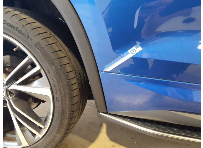
Damage 4: Door - rear right side: Brightware - lower - Scratched - Smart repair
