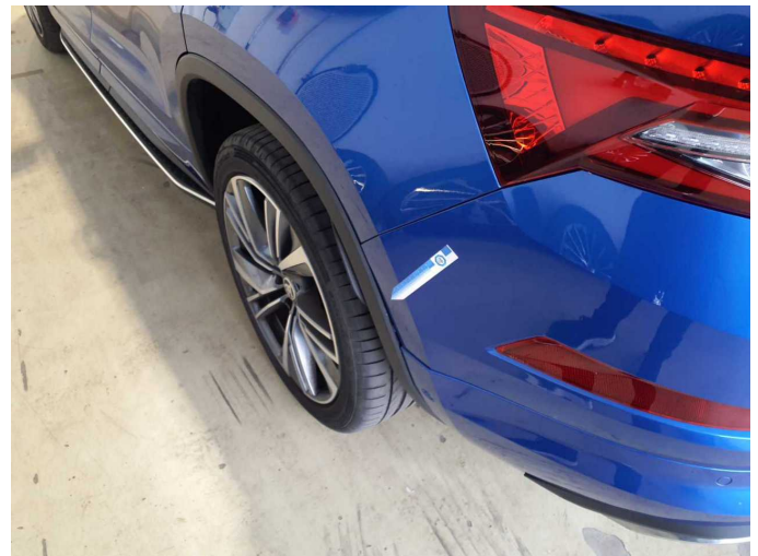
Damage 8: Side panel - rear left side: Wheel well extension - Deformed - Replace
