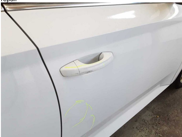
Damage #9: Door - front right side: Door handle - outside - Scratched - Repair and paint
