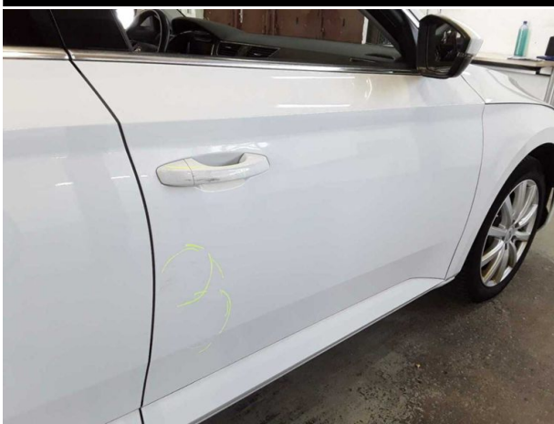
Damage #10: Door - front right side: Door - Dent / paintcoat damage - Repair and paint
