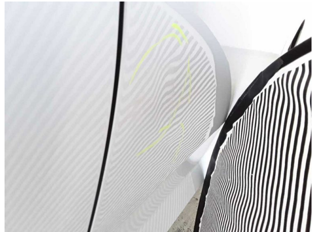
Damage #10: Door - front right side: Door - Dent / paintcoat damage - Repair and paint
