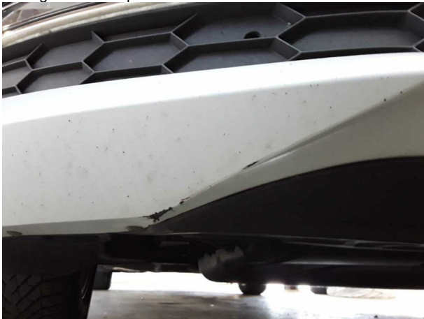
Damage #8: Front bumper: Front bumper - Scratched - Smart repair
