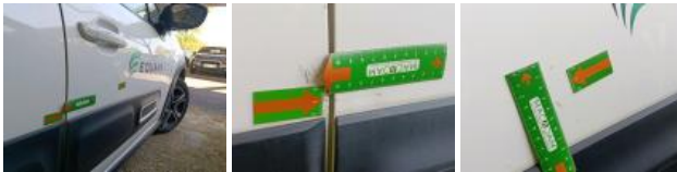
Door RR, Dent(s), Repair and paint (complete)
