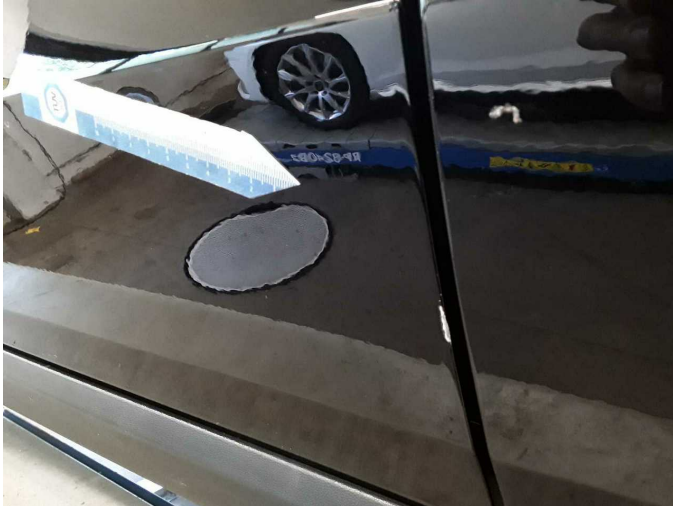
Damage 4: Door - front left side: Door - Scratch(es) - Smart repair
