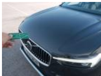
Bonnet, Dent(s) and scratch(es), Repair and paint (complete)
