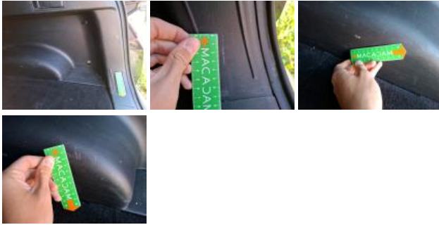
Tailgate / Boot, Dent(s) and scratch(es), Repair and paint (complete)
