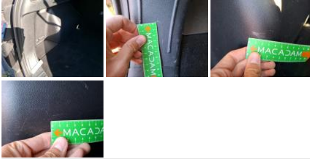
Internal boot lining R, Scratch(es), Replace
