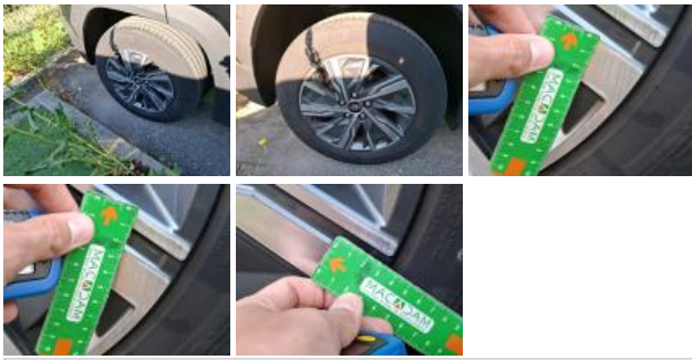
Tyre RR, Out of tolerance, Replace
