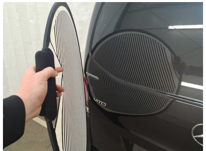
Damage 3: Boot lid / rear door: Boot lid - dent(s) - Repair and paint
