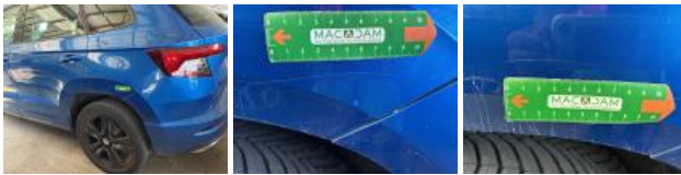
Door RL, Dent(s), Repair and paint (complete)
