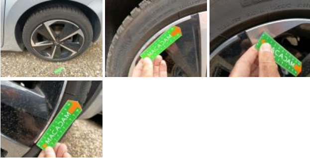
Tyre FR, Out of tolerance, Replace
