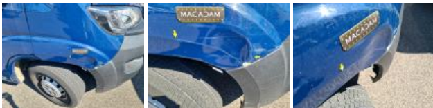
Side repeater R, Broken, Replace
