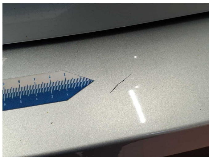
Damage 5: Rear bumper: Rear bumper - Scratch(es) - Paint
