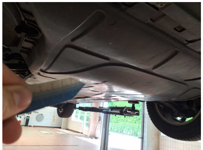
Damage 4: Body: Underbody panelling - Broken / torn - Replace
