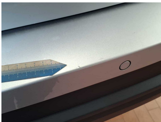
Damage 5: Rear bumper: Rear bumper - Scratch(es) - Paint
