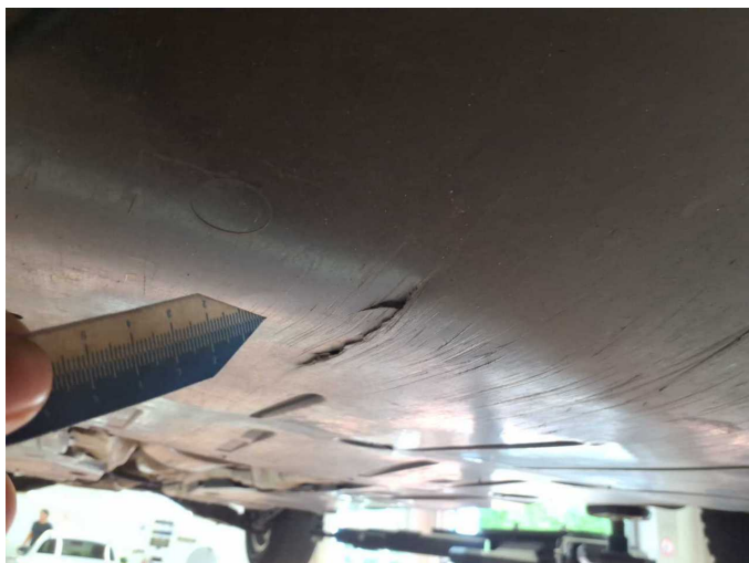
Damage 4: Body: Underbody panelling - Broken / torn - Replace
