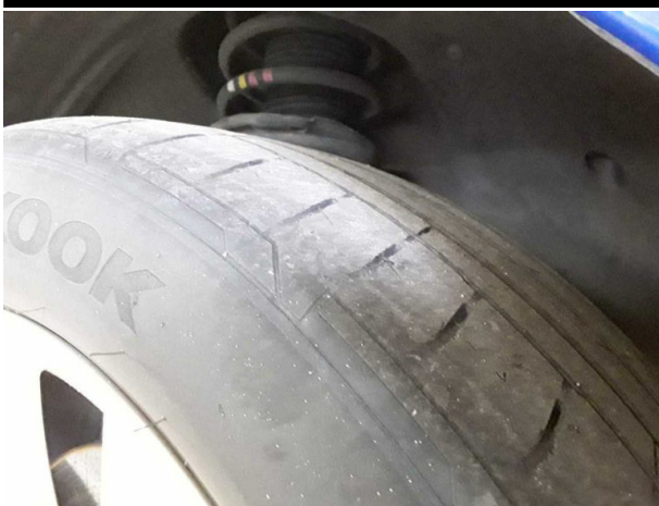
Damage #6: Measurement: Undercarriage - Malposition - Set / adjust
